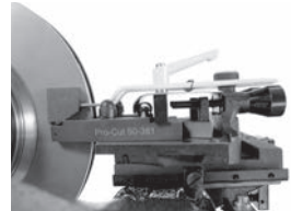
The chip deflector reduces vibration and should be used on EVERY cut.
