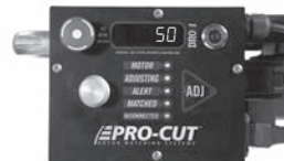
DRO computer in READY mode displaying speed.
