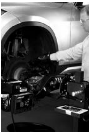
STEP 4. Technician sets cut depth.
